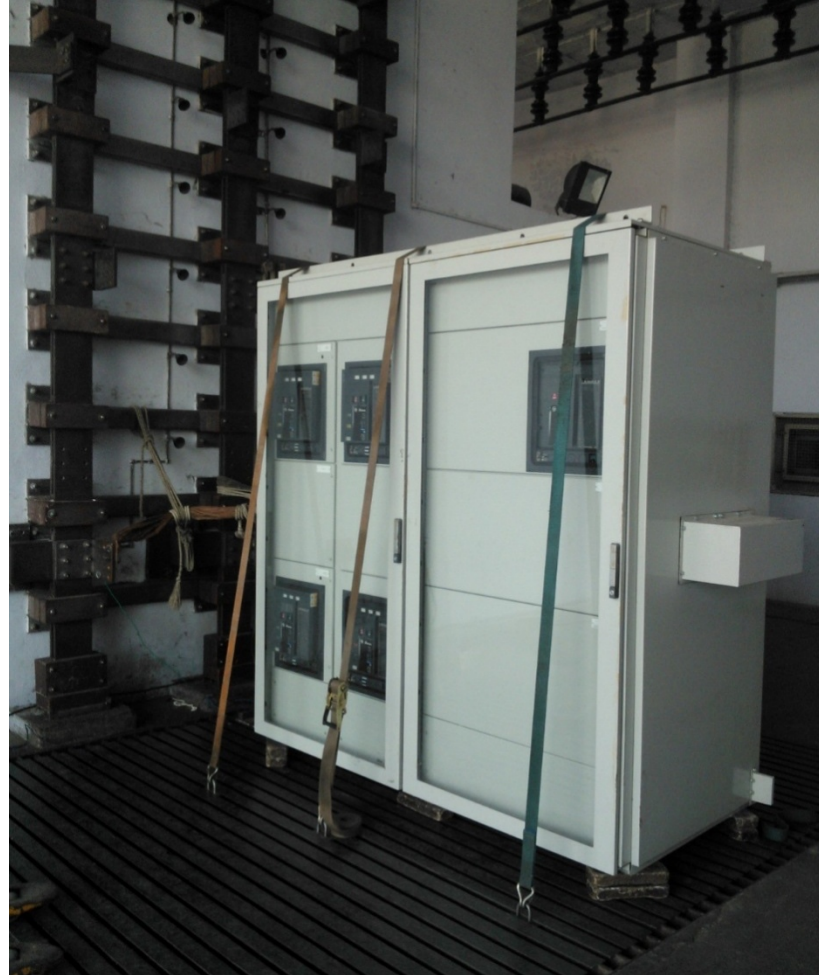
Short circuit test board
